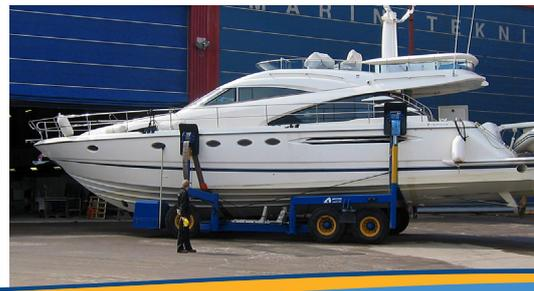
The SUBLIFT 25t is a workhorse used by marinas and boat clubs with a wide range of boats. It is equipped with slings on two pairs of hydraulic lifting arms. The hoist is designed for up to 25 ton boats.
